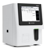
The DH36 is a excellent performer, fit for the demands of the modern laboratory. With 21 reportable parameters and 3 histograms for WBC, RBC and PLT, the analyser also boasts an intuitive user interface, supporting bi-directional LIS. The compact design and built in lyse compartment save space, and it requires only a 9µl sample volume for analysis.
